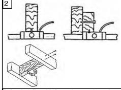
Before installing this fan make sure the outlet box is properly installed to the house structure. To reduce the risk of fire, electric shock, or personal injury, mount to outlet box or supporting system acceptable for fan support. (Mounting must support at least 35 lbs. (16 kg.)).
